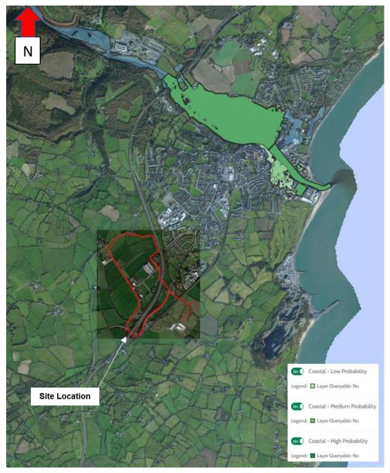
Insert 4.4 Extract from CFRAM Coastal Flooding Map for the Site Area (CFRAM, 2022).
